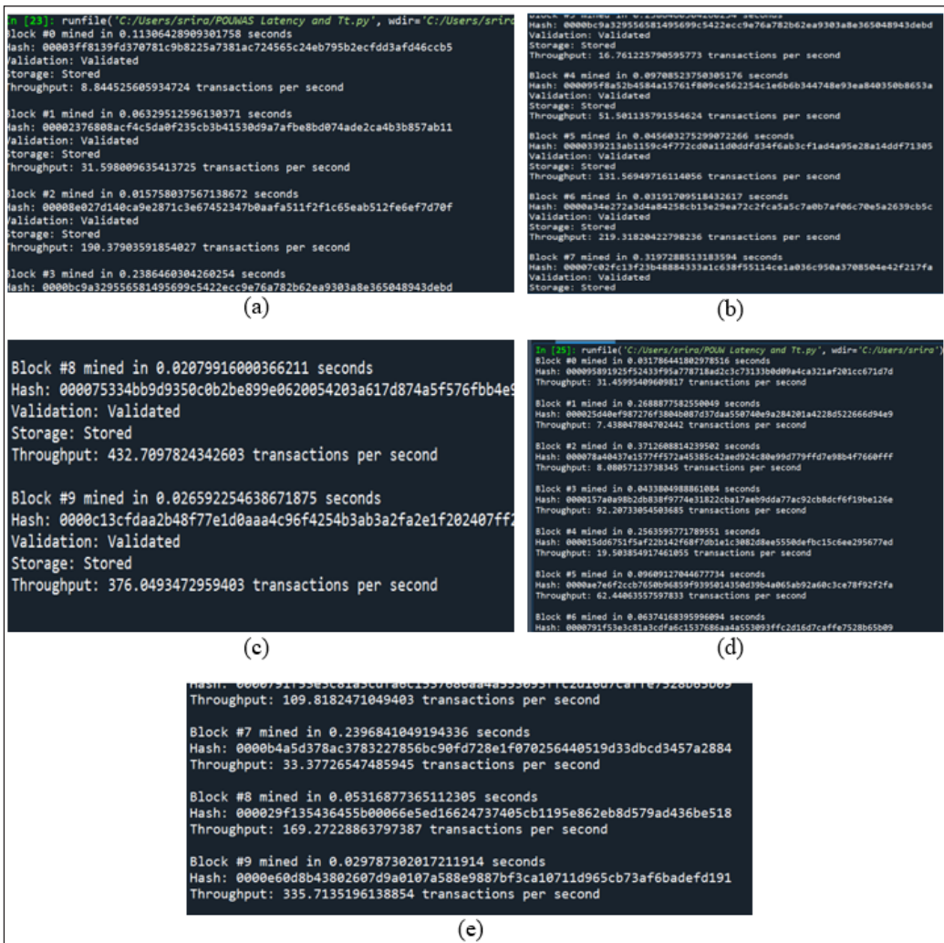
Figure 7. Latency, and transactional throughput: (a), (b), (c) Proposed PoUWAS; (d), (e) existing PoW
